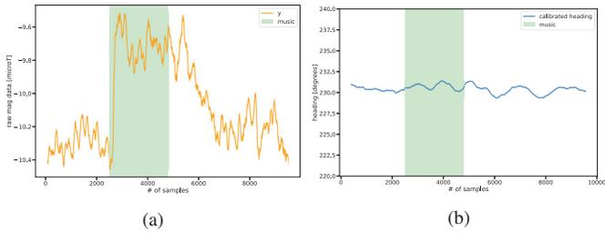
Fig. 2: Impact of audio streaming on calibrated magnetometers.
