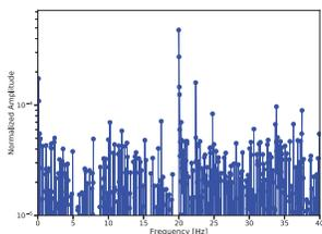
Fig. 3: FFT of the magnetometer traces while playing (on high volume) pure tones at  $20Hz$ .
