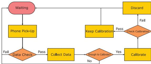
Fig. 6: Auto-Calibration procedure.
