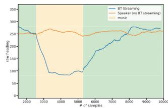
Fig. 4: Impact of BT streaming and speaker on the heading estimated by the raw magnetometer.
