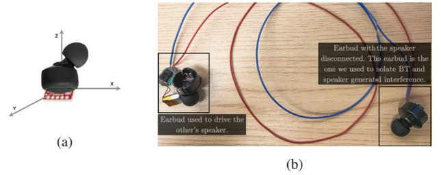
Fig. 1: Basic system setup (Figure 1a) and setup used to isolate the interference generated by BT streaming and speaker (Figure 1b).
