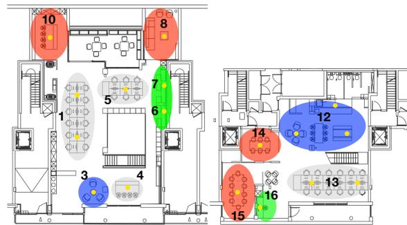
Fig. 3. Floor plans of the first floor (left) and lower ground floor (right) of the office space studied in this work. The yellow circles represent the location of the static BLE beacons. The coloured shadows represent the category of the locations.
