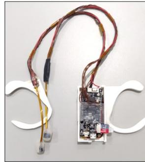
Fig. 7: Earable prototype with IMU and PPG in each earbud.
